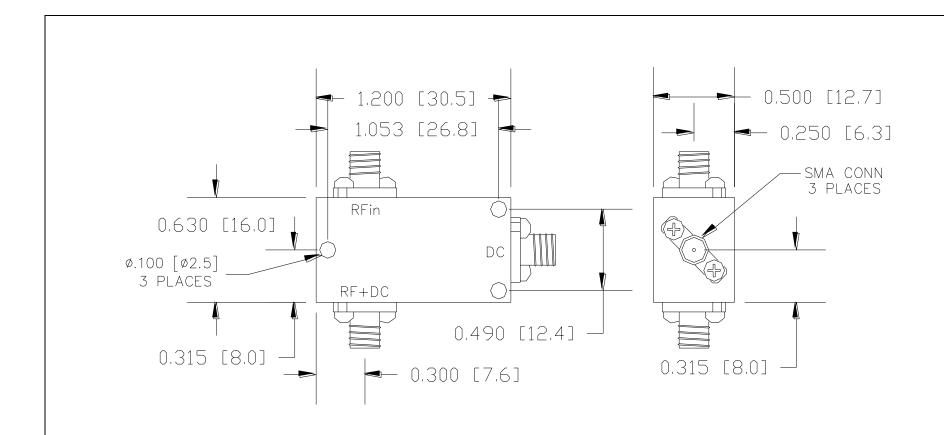
Frequency Range: 300 - 18000 Mhz Insertion Loss: dB Max 1.5 Isolation: 30 dB Тур 25 dB Min **Current Amps:** 0.5 Amp Max **VSWR** Input: 1.60:1 Max Vdc: 50 Vdc Max
