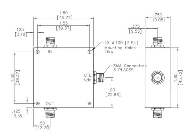
Frequency Range: 0.8 - 1.1Mhz Insertion Loss: 3.5 dΒ Max Phase Shift: 360 Min degree Vdc Control Voltage: 0-20 Max **VSWR** Input: 1.80:1 Max **VSWR Output:** 1.80:1 Max Input Power: +5 dBm Max Input power is rated for load VSWR better than 1.20:1
