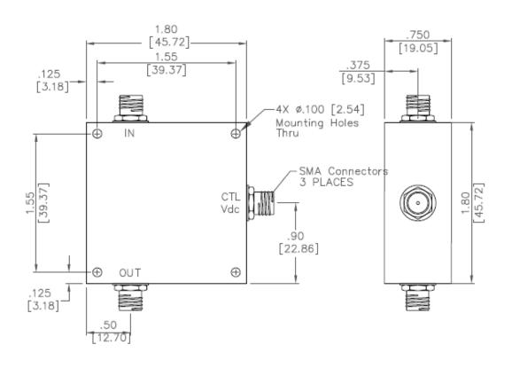
Frequency Range: 70 - 140Mhz Insertion Loss: 3.8 dΒ Max Phase Shift: 360 Min degree Vdc Control Voltage: 0-20 Max **VSWR** Input: 1.80:1 Max **VSWR Output:** 1.80:1 Max Max Input Power: +5 dBm Input power is rated for load VSWR better than 1.20:1
